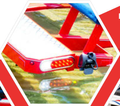
RETRACTABLE TIEDOWNS & STOP, TURN, REVERSE LED LIGHTS
