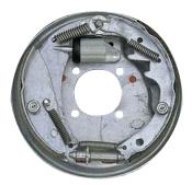
Fig 13: Hydraulic Drum Brakes
