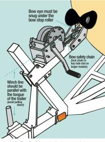
Fig 6: Proper winch operation
