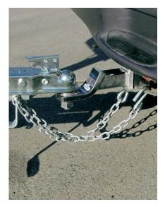
Fig 3: Proper attachment of the safety chains is essential to trailer safety. Note how the safety chains are crisscrossed.
