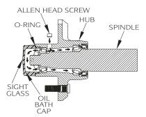
Fig. 17: Oil Bath Hub Lubrication System.
