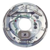
Fig 15: Electric Brakes
